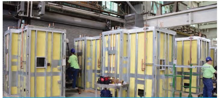
*When the outer shells are completed they are moved off the leveling plates to the finishing area where the plumbing fixtures, electrical, tiling and all other is work is done to complete the bathroom pod.*
