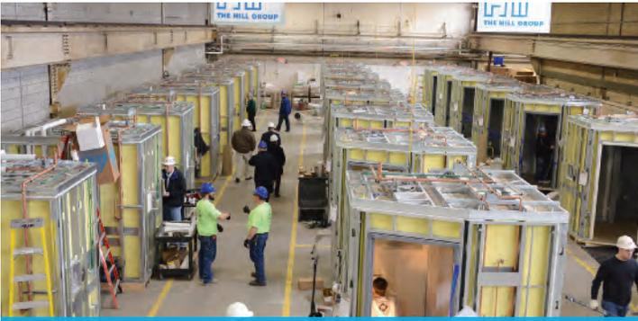
*There is plenty of floor space in Hill's assembly shop to complete all the plumbing and other details and to store the finished pods ready for delivery.*
